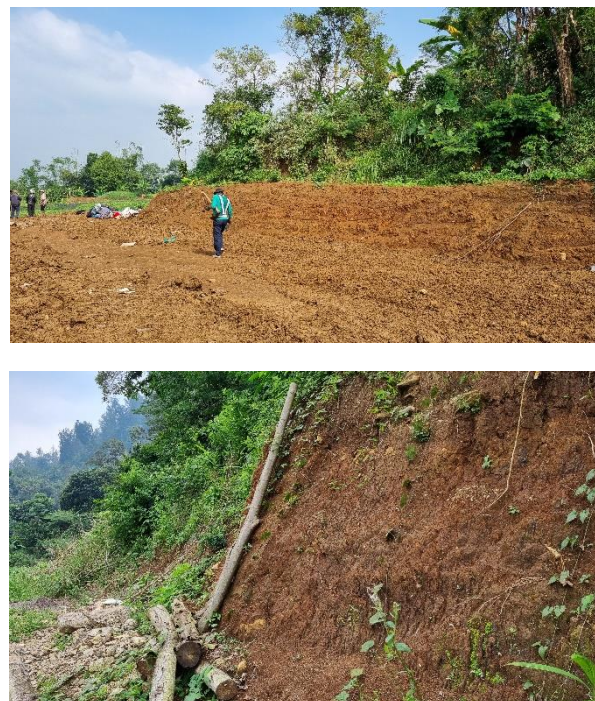
Fig. 1. Typical yellowish to dark brown residual soil and highly weathered breccia in the landslide area, exposed in the middle of the Cijedil Landslide (top) and in the crown area of Cugenang landslide (bottom).
