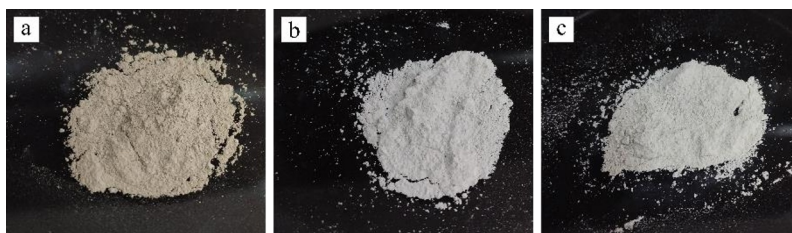
Fig. 1. The visual appearance of (a) as-synthesized SnO 2 powder samples, and after calcination at (b) 300 and (c) 500 °C.
