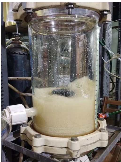
Fig. 2. Experimental installation with a single tray and on bubble-cap.
