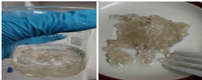
Fig. 7. \text{Fe}_2\text{O}_3 @ \text{MnO}_2 (core-shell) NPs Entrapped by calcium alginate beads.
