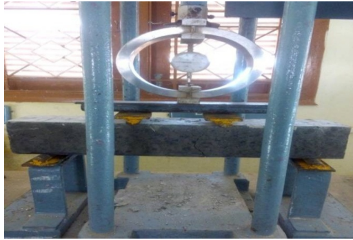
Fig 3. Test Set-up for Flexural Strength Test
