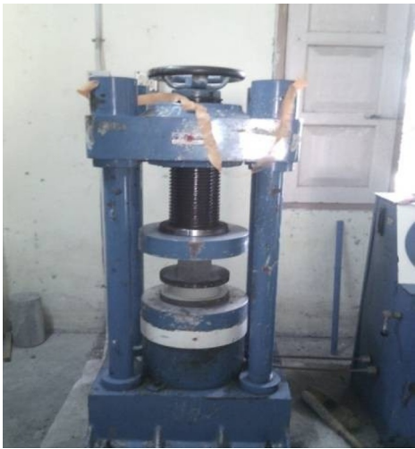
Fig 2. Test Set up for Compressive Strength Test
