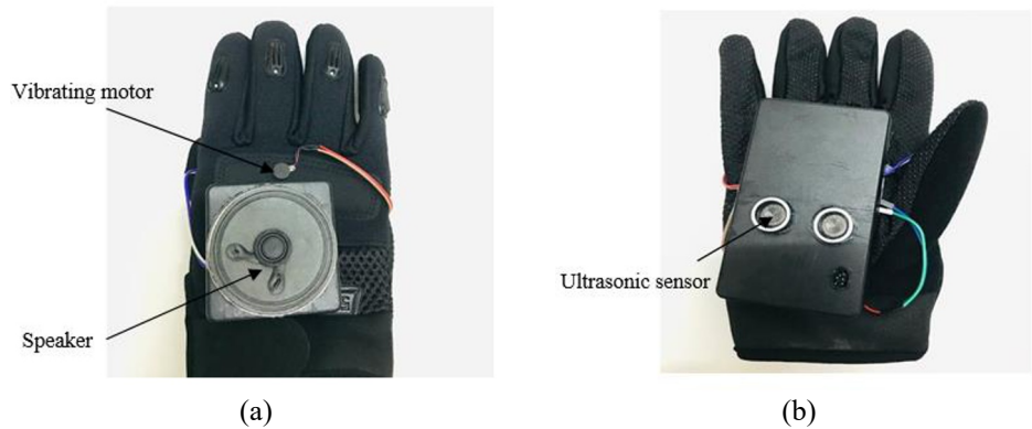
Fig. 7. Prototype of the proposed system. (a) Top of the glove and (b) the palm of the glove
