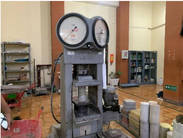
Fig. 2. Compressive strength with compressing testing machine.
