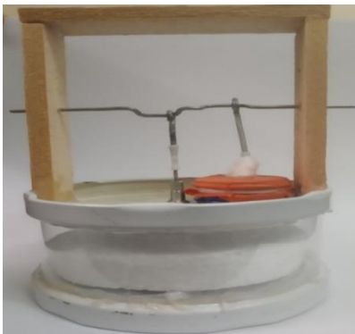
Fig. 4. A practical Stirling engine operating at a low temperature difference.
