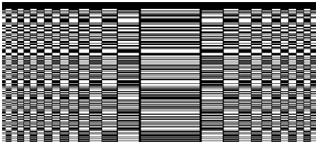
Fig. 16. Radio hologram of a point target forming by BPSK signal.
