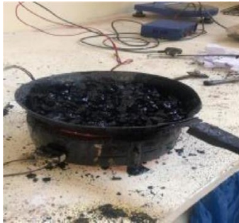
Figure 6: Mixing of Bituminous Material
