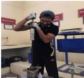
Figure 7: Compaction of the Mix
