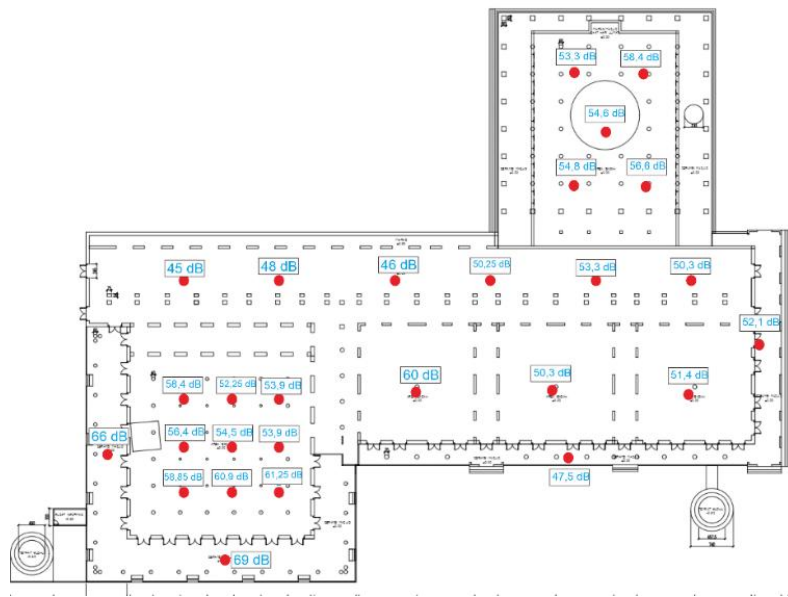
Fig. 3. The Background Noise of Sunan Ampel Great Mosque shows the highest level is in the pyramidal roof area, and the lowest level is in the flat roof area.
