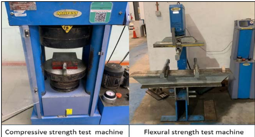
Fig. 2. Machine used for compressive strength test machine and flexural strength test.
