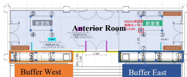
Figure 7. Locations of temperature and humidity sensors installed in the anterior room and buffer zones at multiple heights (FL+100 to FL+4,100)
