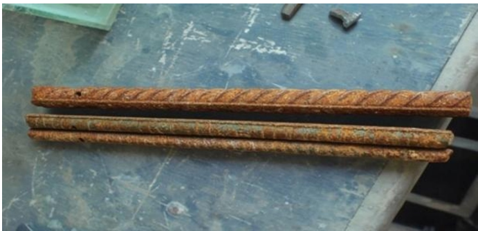
Fig. 10. TMT-Rod with Nano- Silica and Epoxy Coating
