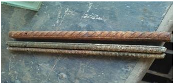
Fig. 7. Steel Rods in 3% NaCl Solution: Before and After Corrosion Exposure.
