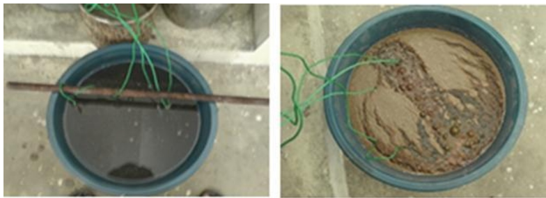
Fig. 7. Steel Rods in 3% NaCl Solution: Before and After Corrosion Exposure.
