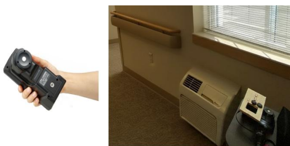
Fig. 1. Spectral data collection setup with CL500-A spectrophotometer in the nursing home location of the study.
