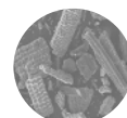
Fig. 1. SEM image of rice husk material obtained for a magnification of 50\times .
