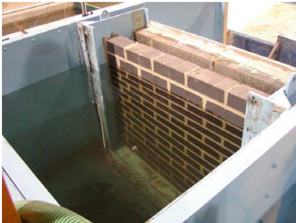
Figure 2. Testing a cavity masonry wall.
