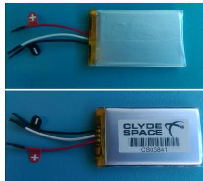
Figure 2. Individual Varta Lithium Polymer Pouch Cell
