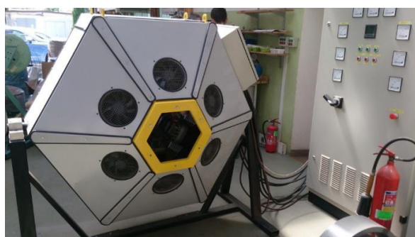
Fig. 3. Laboratory class electromagnetic mill with a diameter of 200 mm used for investigations (by D. Foszcz).
