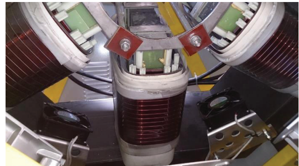
Fig. 1. Electromagnetic field inductor (by D. Foszcz).
