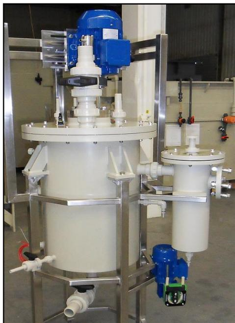
**Fig. 2.** Reactor of 50 dm<sup>3</sup> volume used for regeneration of acidic copper chloride solutions.
