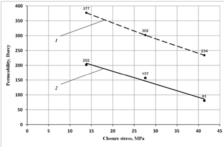
**Fig. 1.** Dependence of the permeability of the fracture wedged with Borprop 20/40 proppant on the closure stress: 1 – initial permeability; 2 – data obtained at the assembled laboratory unit.
