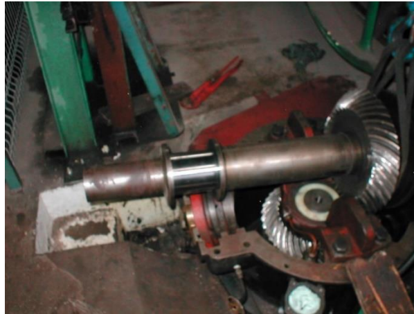
Fig. 3. The toothed intersecting axis gear after the renovation.
