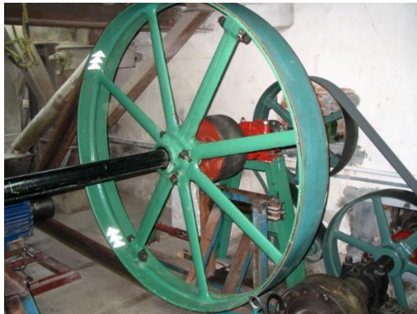
Fig. 5. The modernized belt gear.
