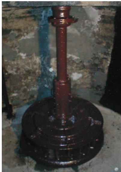
Fig. 1. The 110/170 cm Francis turbine from 1936.
