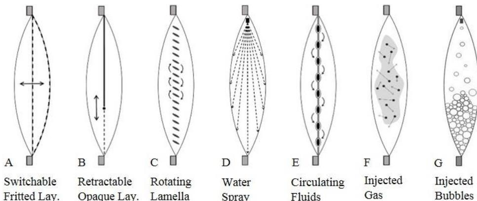
**Fig. 3.** Environmental control mechanisms for multilayer foil constructions.
