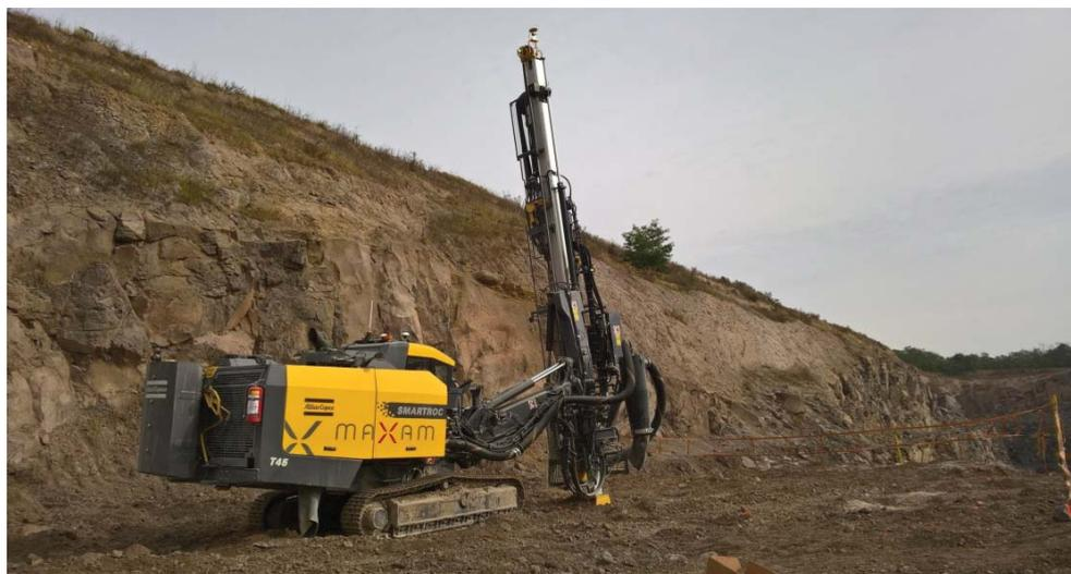
**Fig. 1.** SmartROC T45 drill rig with a GNSS Leica receiver [7].
