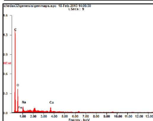
(b) SEM & EDS test of interface between wood and resin-ramie after 5.5 months field test
