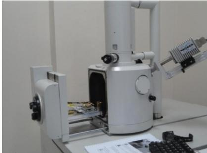
**Fig. 1.** Scanning Electron Microscope (SEM)
