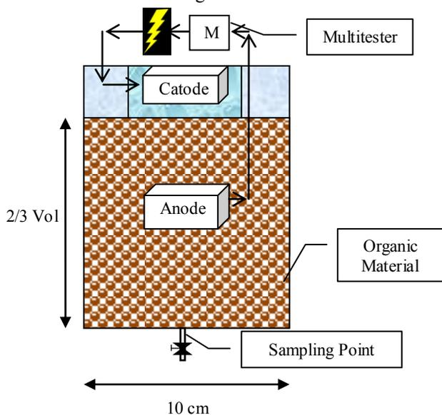
Fig. 1. SMFC Reactor Configuration.
