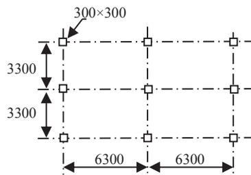
**Fig.2.** The mesh of columns
