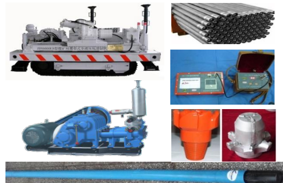
Fig 1 Directional drilling equipment of fire abnormal detection
