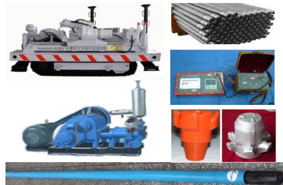
Fig 1 Directional drilling equipment of fire abnormal detection
