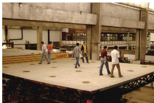
Figure 3 Model Test under Human-induced Vibration
