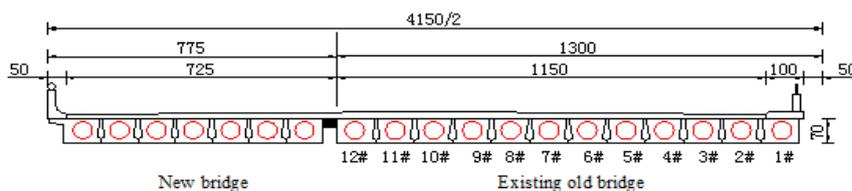
**Figure 1** The Half Cross- section of Superstructure (unit = cm)
