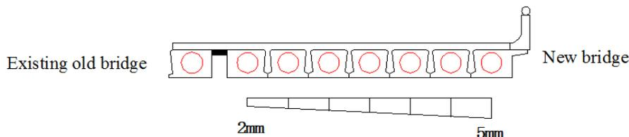
**Figure 5** Foundation Settlement of Widening Structure
