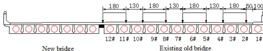
**Figure 4** Distribution Method of Vehicle Load (unit = cm)
