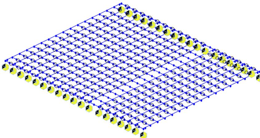
**Figure 2** Space Grillage Model of Superstructure
