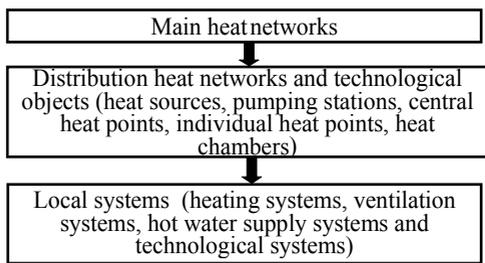
Fig. 1. Hierarchy of calculation schemes of HSS.
