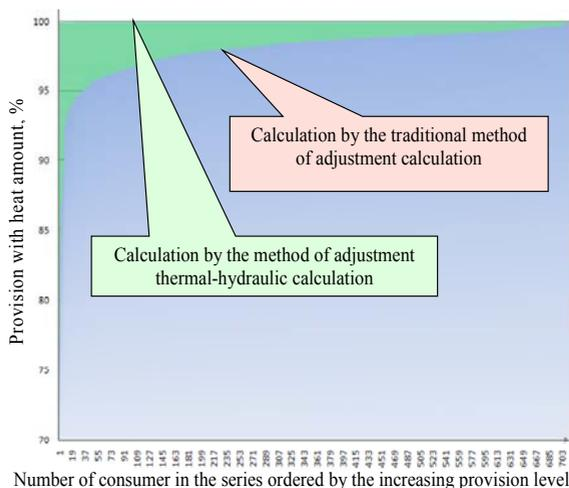
Fig. 3. Graph of consumer provision with heat load.
