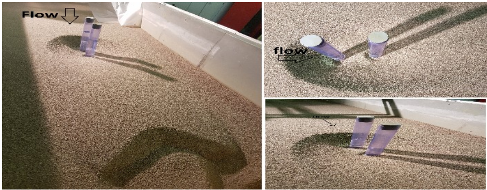
Fig. 1. Eroded sediment bed around the piers after the experiment at the equilibrium state ( \theta = 0^\circ )
