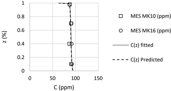
**Fig. 4.** Vertical concentration distributions at MK10 (squares) and MK16 (circles). The gray line represents the Rouse profile fitted on the concentration values. The black dashed line corresponds to the predicted Rouse profile considering the flow conditions and the main mode of the LISST PSD
