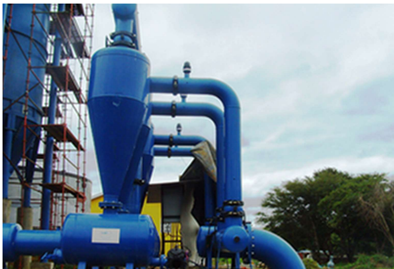
Fig. 1. The outside appearance of hydrocyclones.
