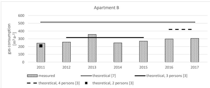
Fig. 4. Gas consumption for DHW in apartment B .
