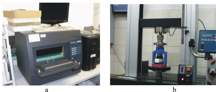
Fig. 3. Measuring apparatus used in the tests: a) NETZSCH plate apparatus, b) universal strength testing machine QCTECH.
