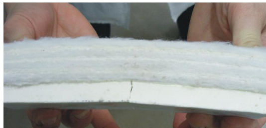
Fig. 6. View of an example sample after the bending strength test.
