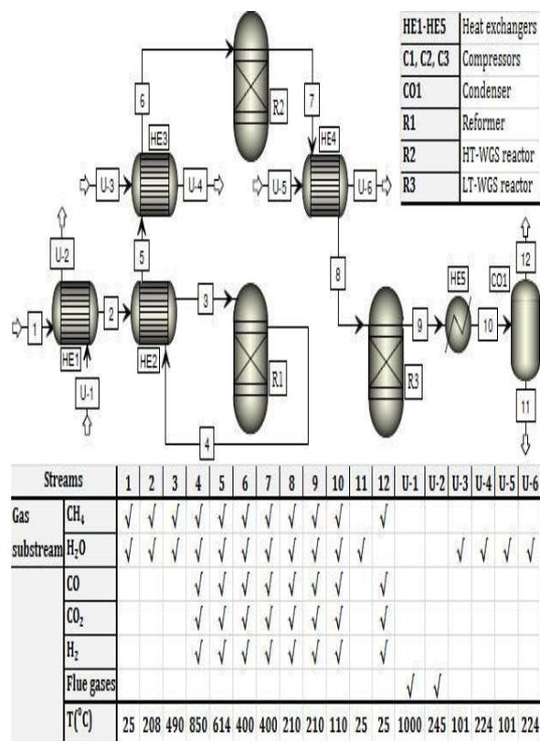
Figure 1. Steam Methane Reformation Process Working Principle [38]
