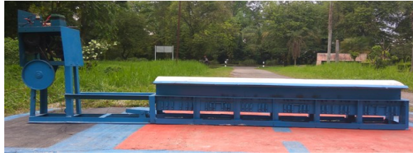
Fig. 1. Power generation apparatus using speed bump.
