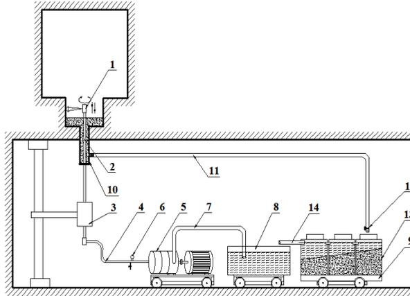
**Fig. 2.** Diagram of the experimental monitor plant: 1 – monitor head, 2 – monitor barrel, 3 – monitor unit, 4 – high-pressure hose, 5 – pump, 6 – manometer, 7 – water pipe, 8 – water tank, 9 – container platform, 10 – production hole preventer, 11 – pulp line, 12 – discharge device, 13 – hydrodisintegrated products, 14 – water overflow.
