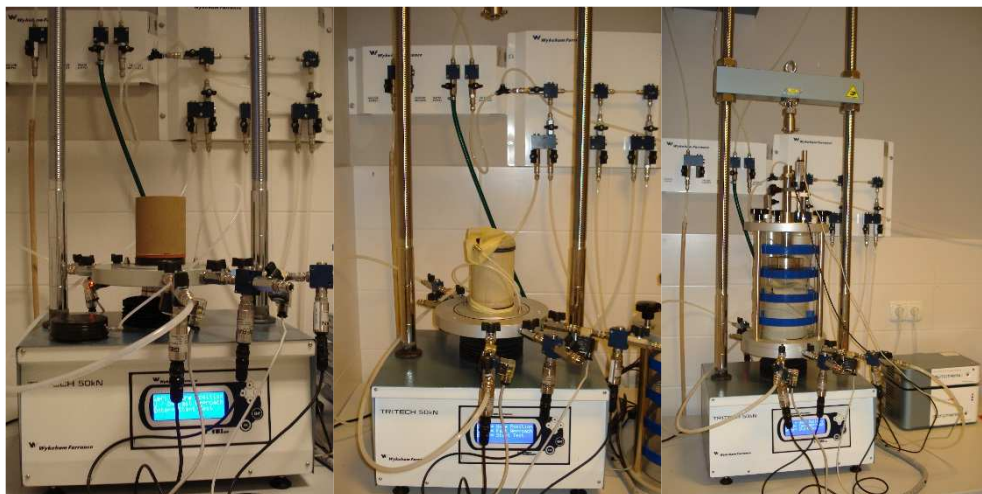
Fig. 4. The stages of sample preparation for permeability coefficient testing.
