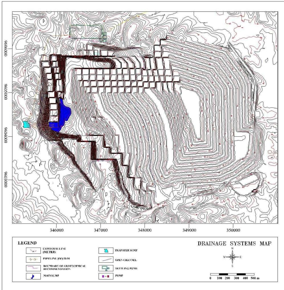
**Fig. 3.** Design map of coal mine drainage system based on water catchment areas, rainfall data, runoff discharge, and information on rain intensity/frequency.
