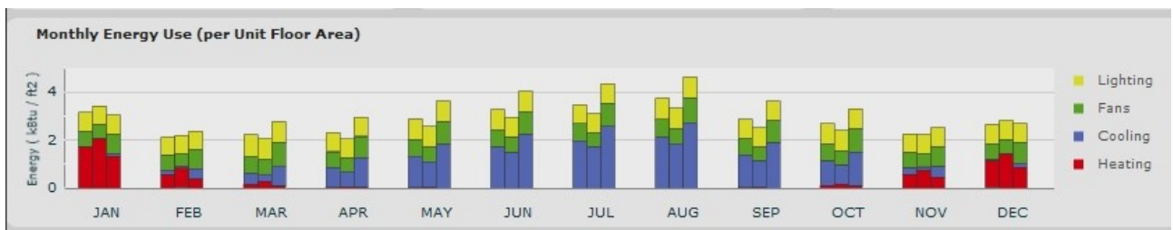
Fig. 6. Monthly energy use per room floor area unit for the 3-person case, in the following order: screen, fine screen, no-shading .
