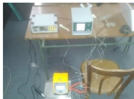
Fig. 6. Thermocouples calibration bench.
