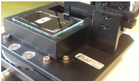
**Fig. 2.** Stereoscopic image calibration kit for MicroPIV.
