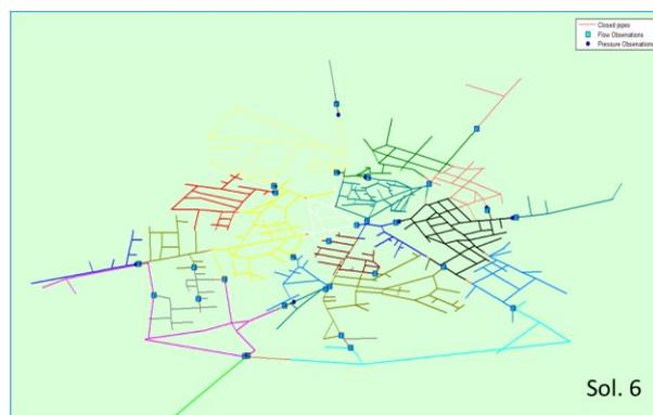
**Fig. 10.** DMA design solution 6.
