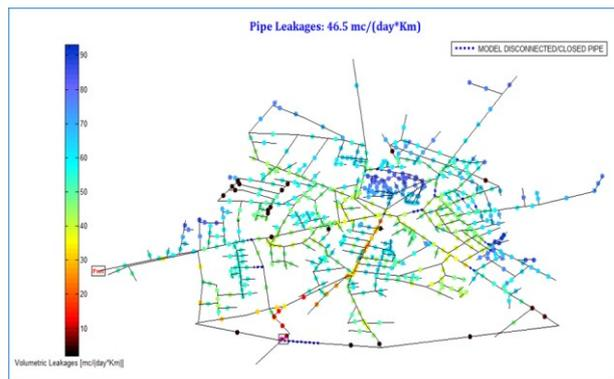
**Fig. 14.** Linear leakages in DMA design solution 3.
