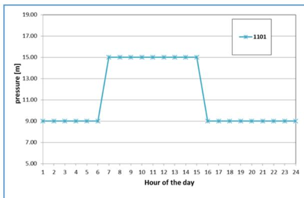
**Fig. 2.** Original pressure settings of the *local* PRV.
