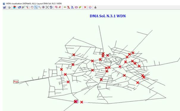
**Fig. 11.** Closed gate valves in DMA design solution 3.
