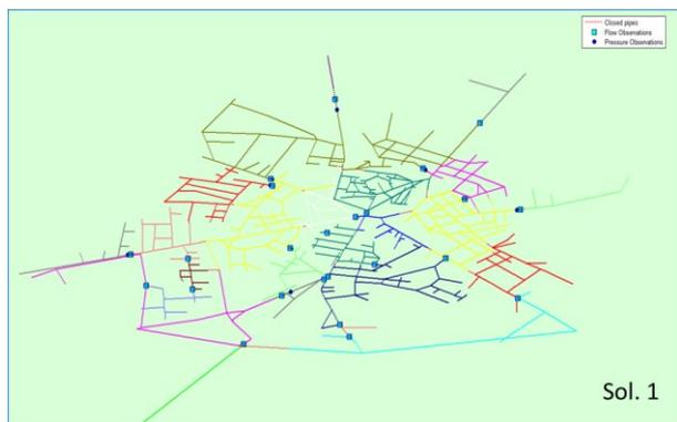
**Fig. 5.** DMA design solution 1.
