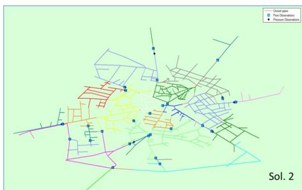
**Fig. 6.** DMA design solution 2.
