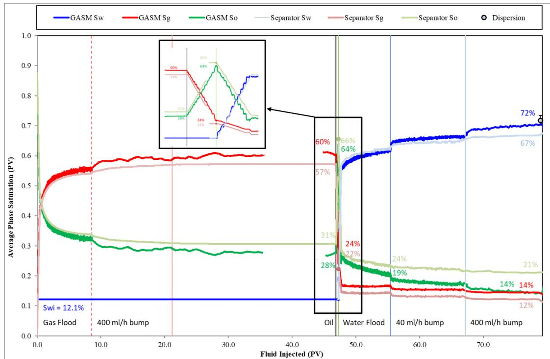
**Figure 5.** Saturations during Coreflood 2
