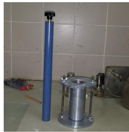
Fig. 2. Compaction mold and special hammer to apply standard proctor energy used in this study
