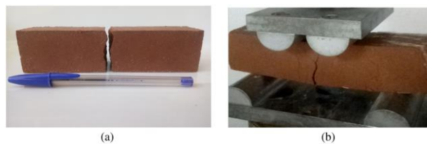
Fig. 4. Rupture mode (a) cemented sand – fragile (b) fibre-reinforced cemented sand – ductile
