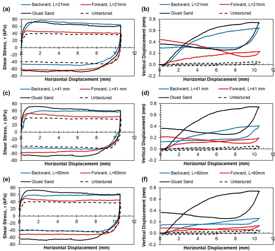
**Fig. 2.** Mobilized shear stresses and associated vertical displacements from tests on Hostun sand.
