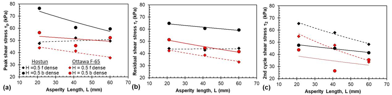
**Fig. 4.** Mobilized shear stresses: (a) Peak, (b) residual, and (c) 2<sup>nd</sup> half-cycle.
