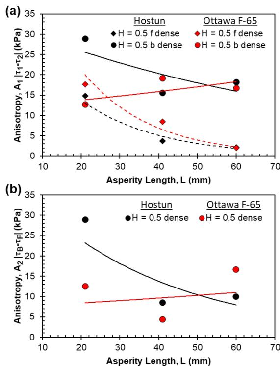
**Fig. 5.** (a)  $A_1$  and (b)  $A_2$  frictional anisotropy parameters from tests on Hostun and Ottawa F-65 sands.
