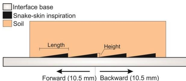
**Fig. 1.** Interface shear specimen configuration
