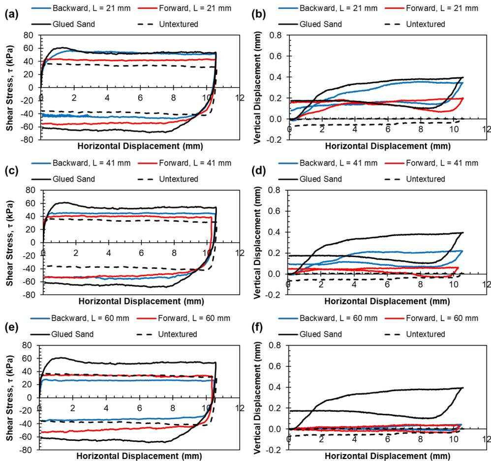
**Fig. 3.** Mobilized shear stresses and associated vertical displacements from tests on Ottawa F-65 sand.
